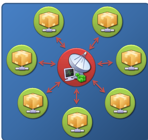
Figure 1: Star CnC topology with direct communications between the central command hub and each bot agent
